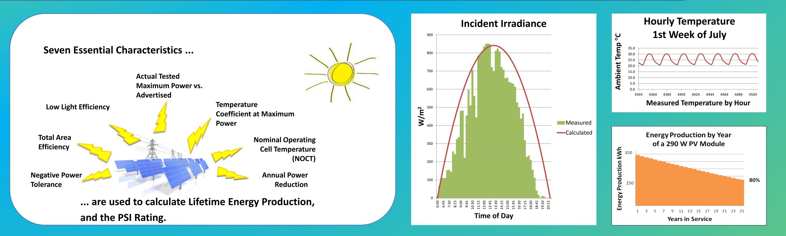
These models of irradiance and temperature are applied to the seven key module characteristics, and the impact on each one is combined without weighting to obtain the 25 year LEP. Degradation over time is based on warranty terms, not accelerated testing. We normalize the energy value using the total irradiation accumulated per square meter in 25 years. In this way, PV modules can be compared as if installed side-by side irrespective of orientation, tracking configuration or inverter choice.
