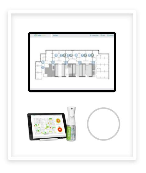
Professionals release tracers in designated test areas for dispersion throughout a building and air ducting. Air and surface samples are collected and tested at selected points and time periods.
